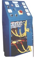
Custom built power supplies can be manufactured to your exact requirements. These can be single or three phase input, and AC or DC output. The output can be fixed voltage, or variable voltage: variable output may be adjustable in fixed steps or be continuously variable. The output can range from a few volts at several thousand amps to several thousand volts at a few milliamps.
