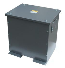
Our transformers in this range are suitably protected by a sheet metal case. They are normally wall mountable up to 6kVA and floor standing above this rating, but a portable style is also available. Many requirements are for low voltage tools or lighting working at 24V or 110V to be fed from mains supplies of 230V or 400V. The above voltages are not exclusive and other inputs and outputs can be accommodated on request.
